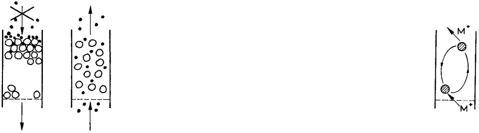
Fig. 1. A packed column will be blocked by particles, a fluid bed will not.
